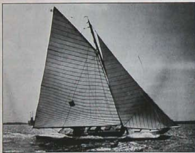
With the main eased off so it's partly backwinded by the jib, these boats could carry full sail even in a blow.
